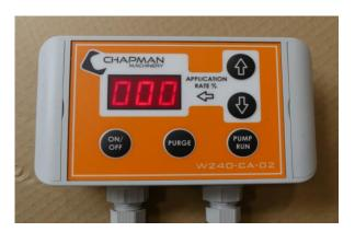
**ON/OFF:** Switches the control box on or off. When switched on, the applicator roller will run continuously.
