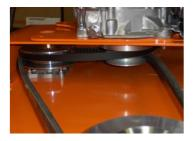
7. Re-tension belts using 17mm spanner on tension bolt below engine
