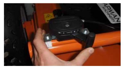
With the throttle at full choke, pull the plastic part of the cable upwards, and tighten the retaining bracket when the choke lever just touches the plastic topped adjuster screw. Test for correct start / stop operation.
