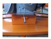
3. Place belt over pulley 1 and 2 on lowest groove
