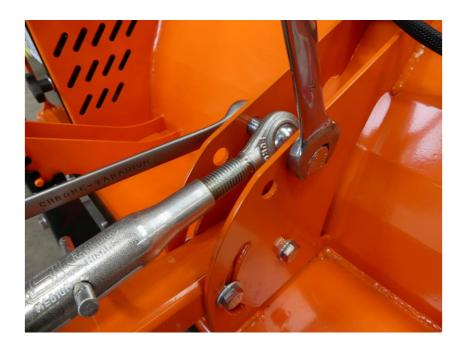
**Do not overtighten the bolts**, they only need to be just 'nipped' up to allow the drawbar to move up and down when the adjuster is used.
