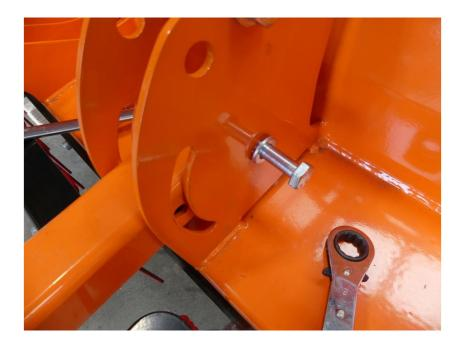
Next, install the other 19mm bolt & nut in through the most forward hole and again, loosely.
