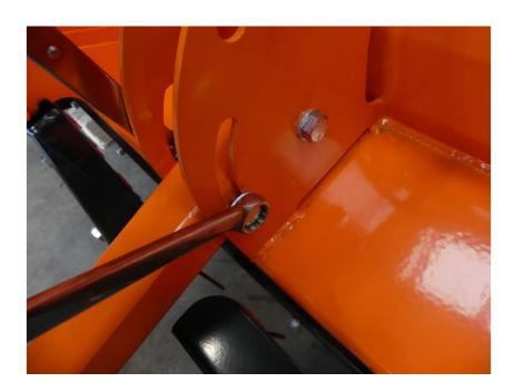
Supporting the weight of the drawbar, lift up until the drawbar adjuster is inline with the last 24mm bolt fitment at the back of the drawbar mount & install. There should be one aluminium spacing bush on each side of the adjuster assembly (not shown in picture).
