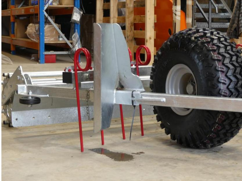
2. With the machine in transport mode remove steel pin and turn the blade to a 90-degree angle (see below) making sure the pin holes are aligned. The perimeter blade can also be used on the left-hand side of the machine.
