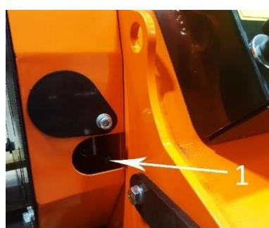
1. Driven Side Rotor Bearing
