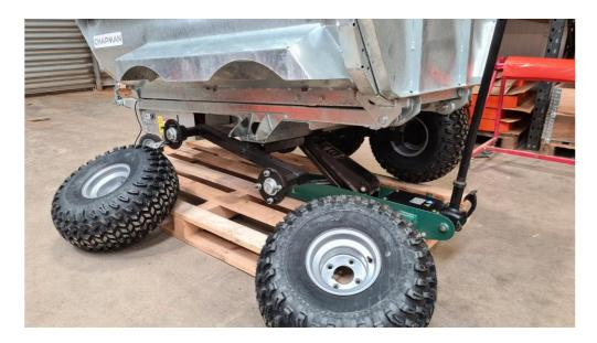
5. Proceed to do the same on the following side, making sure all wheels on both sides are fully tightened. Remove the DT100 from the pallet and proceed with the next steps of Attachment & Set up.
