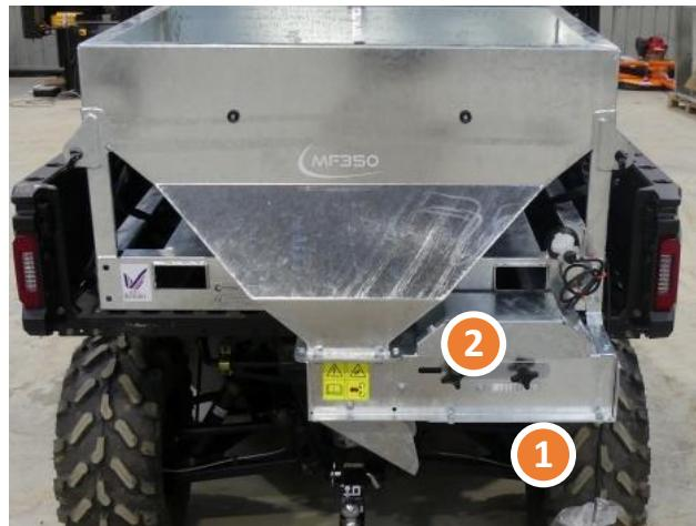
2. You should not need to remove the slide plate to access the sensor, however if you do need to remove the slide plate for access, this can be achieved by unclipping the spring from the slide plate and removing the 5 x bearings and associated bolts which locate the plate. TAKE NOTE OF THE NUMBER OF WASHERS AS THESE NEED TO BE RE-FITTED IN THE SAME ORDER TO ENSURE THE SLIDE MOVES SMOOTHLY.
