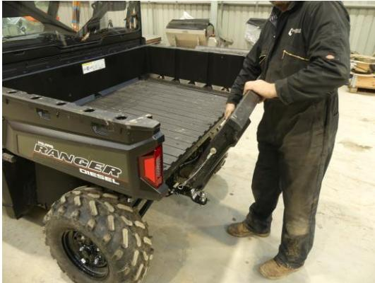
3. Centralise hopper in bed and attach using 4 supplied ratchet straps, 2 straps per side. Ratchet straps must be fitted in a crossing manner as shown below! It is the user's responsibility to ensure the unit is securely fitted in the bed.
