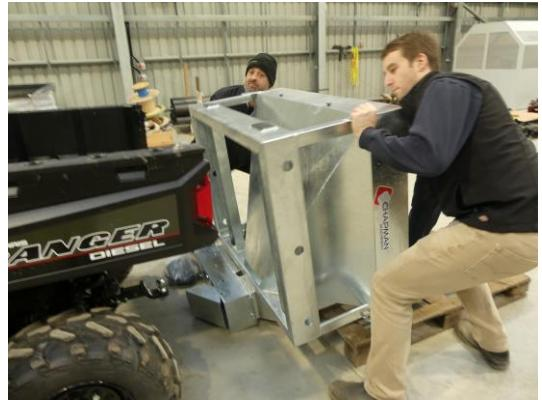
4. Fit the cover support bar to prevent the cover sagging as shown below. Fit tarpaulin cover on top of hopper.
