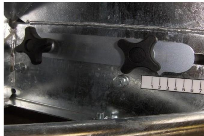
Fill the hopper 50% full of the feed to be distributed. With the machine attached to the towing vehicle and on level ground, switch the control box on and deposit 20 drops of feed into a bucket. Measure the weight of the deposited feed and divide by the number of drops (in this case 20) to give the weight per drop.
