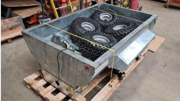
2. Once Drawbar is removed, thread through the hand controller through the end plate
