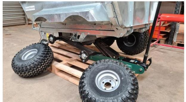
similar (using axle stands where necessary) and attach the wheels. Tighten wheel nuts to 50Nm. CHECK ALL NUTS/BOLTS AFTER 1 HOUR OF USE.
