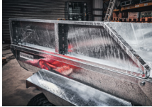
Extension Sides Increases the internal height of the trailer by 300mm allowing for greater capacity.
