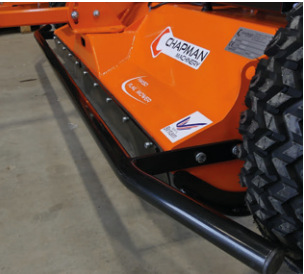
Front Breaker Bar Ensures tall materials (e.g reeds or bracken) feed evenly into the rotor for consistent cutting performance
