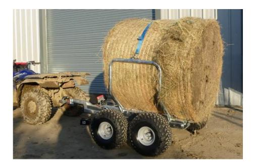
5. As the bale comes "over centre" press the foot latch rearwards again, and keep winding in the electric lift until the cradle is fully resting on the frame. Release the catch and ensure ensure the locking pin has latched securely into place.
