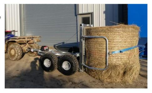
4. Operate the electric lift to load the bale by pressing the "IN" button on the remote or hand control.
